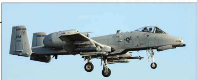
The C-model clearly allows more precision than the A-model: hung with a targeting pod, Maverick and Side-winder missiles.
