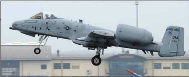
The Thunderbolt II has two engines on the fuselage, but can fly on only one in case the other is hit by the enemy.
