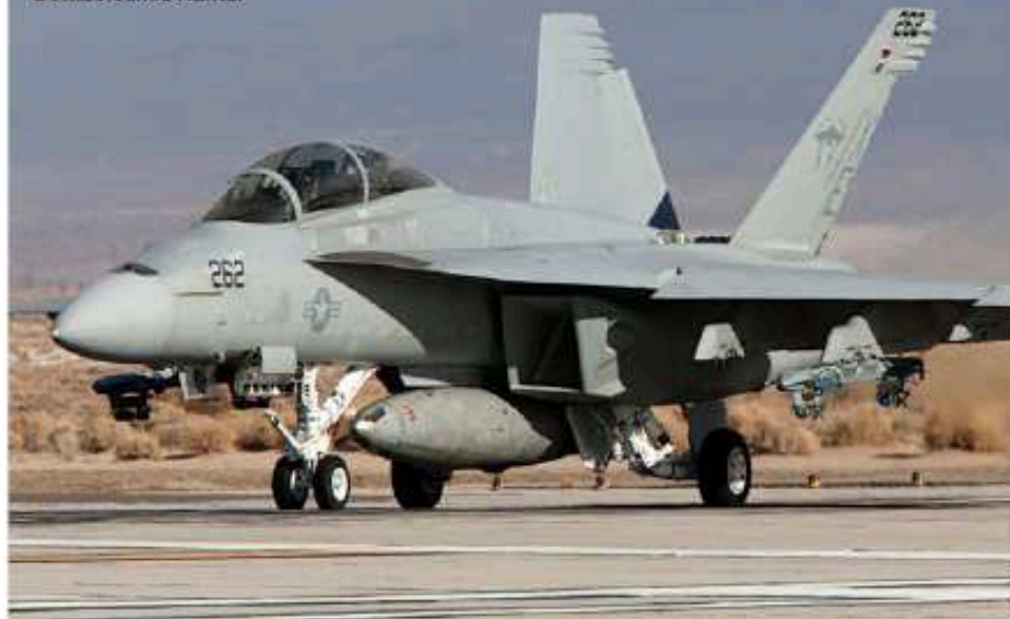
This VX-9 F/A-18F carries an unusual combination of a centerline buddy refueling pod and Mk76 practice bombs. Jamie Hunter
